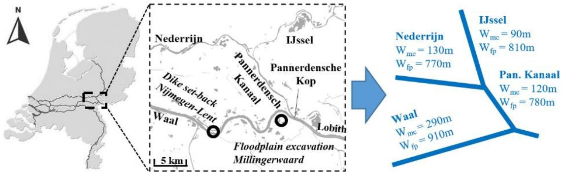
Figure 1. Left: the study area in the Netherlands: the four primary Rhine branches. Indicated with the two circles are two water level reducing river interventions implemented during the Room for the River program. Right: the 1D network schematization of the branches. In this schematization every branch has a uniform compound cross-section with typical main channel width ( $W_{mc}$ ) and floodplain width ( $W_{fp}$ ).
