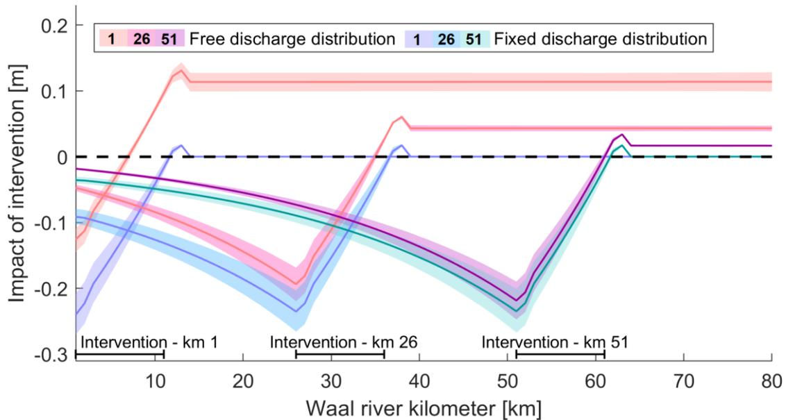
Figure 5. Impacts of interventions with upstream ends at kilometres 1, 26 and 51. Again, the red tones indicate the configuration with free discharge distributions and the blue tones the configuration with fixed discharge distributions.
