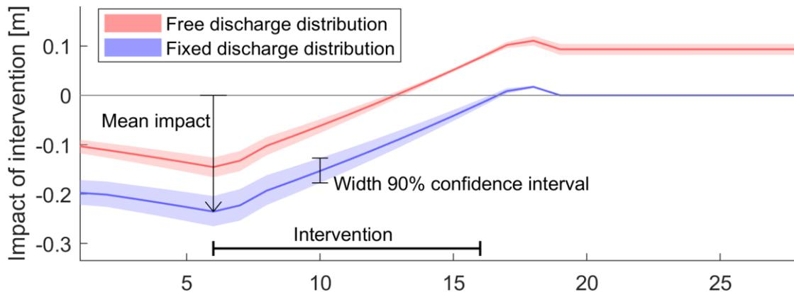
Figure 3. Impact and its uncertainty of an intervention with an upstream end six kilometres into the Waal for an upstream discharge of 16,000 m<sup>3</sup>/s. The shaded areas are the 90% confidence intervals while the continuous lines are the mean impacts. If the discharge distribution is free, the water level reducing effect of an intervention is smaller and a clear downstream increase in water levels occurs.
