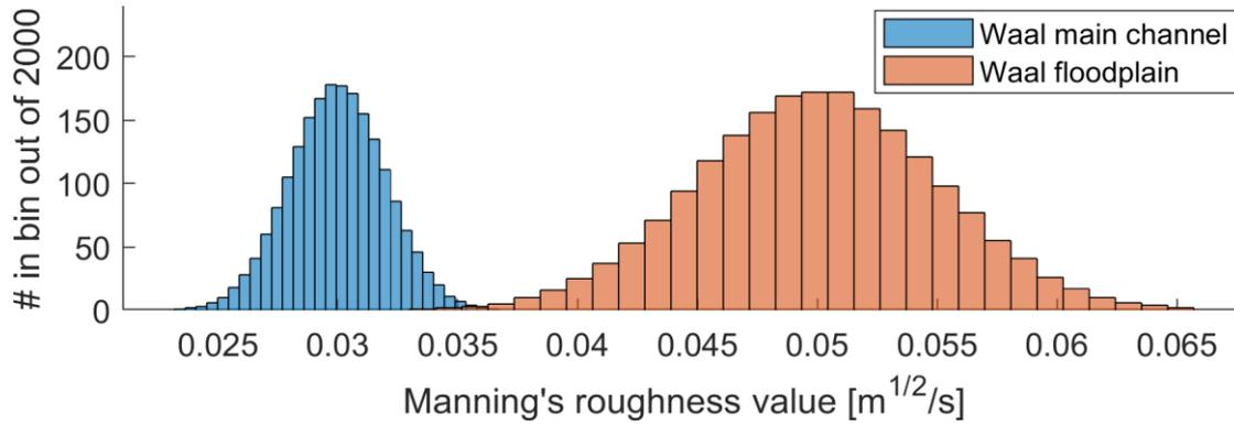
Figure 2. Values of Manning's roughness for the main channel and floodplain of the Waal in the set of 2000 Sobol samples.
