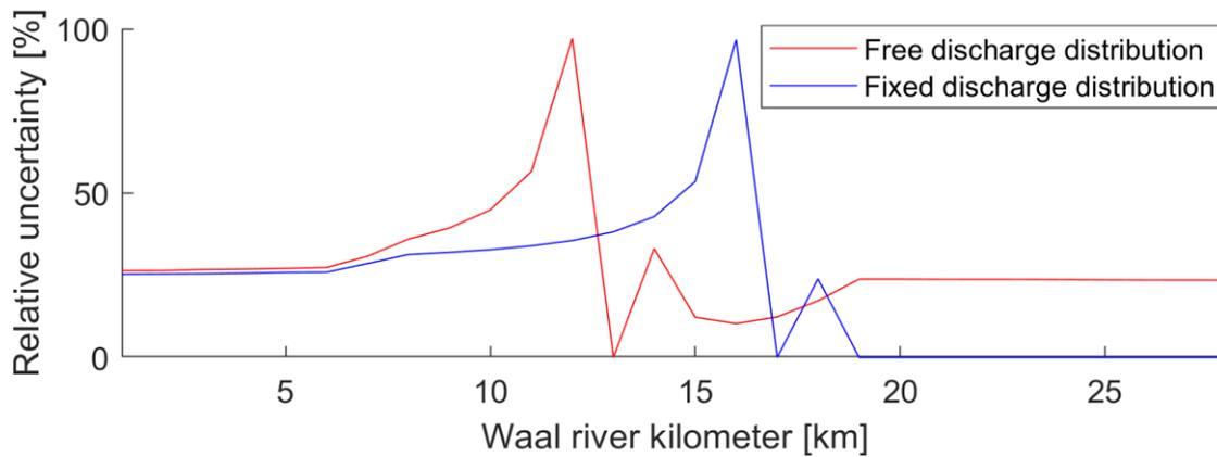
Figure 4. Relative uncertainty of the impact of the intervention in the example case with both a free and a fixed discharge distribution. Having a fixed or free discharge distribution does not influence the relative uncertainty upstream of the intervention. The free discharge distribution has a relative uncertainty downstream that is more or less equal to the relative uncertainty upstream.
