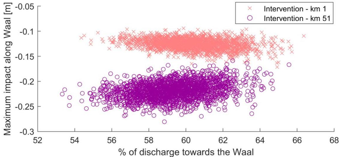
Figure 6. Scatter plot of percentage of discharge towards the Waal versus the maximum change in water level anywhere along the Waal for an intervention at kilometer 1 (crosses) and for an intervention at kilometer 51 (circles). The maximum water level change occurs right at the upstream end of the intervention, i.e. at km 1 and km 51 respectively.
